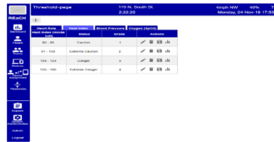
Figure 3:- Thresholds page- Collecting all the health vitals (HR,RR,BP,SPO2) ranges and assigning a grade to each health vital parameter.
